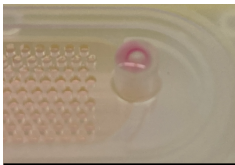
Figure 1. Picture of a trapped air bubble at the inlet
